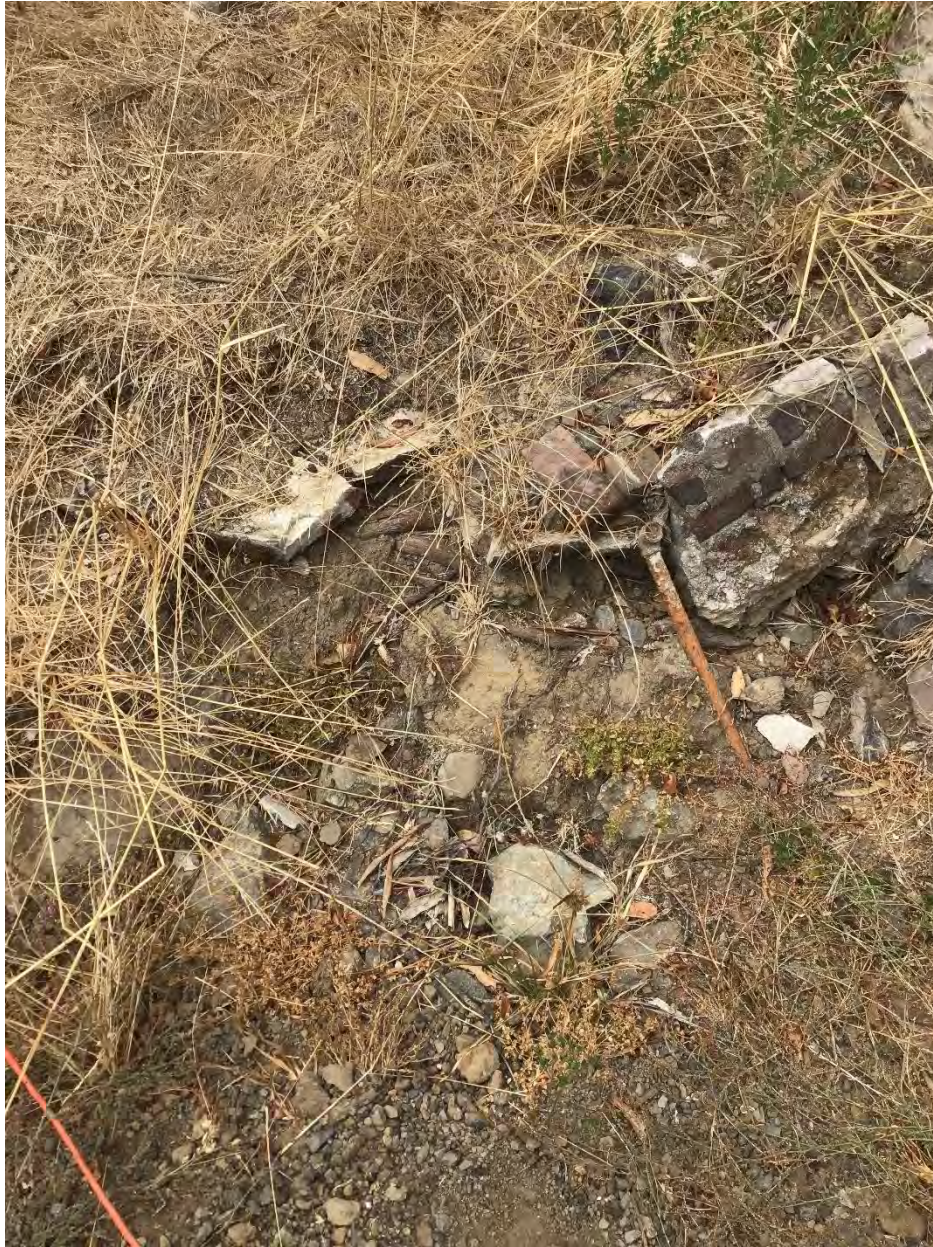
Photo 2. OHWM2 sampling point in ephemeral drainage ES1. OHWM indicators observed included break in bank slope and vegetation stripped from active areas of the channel.
