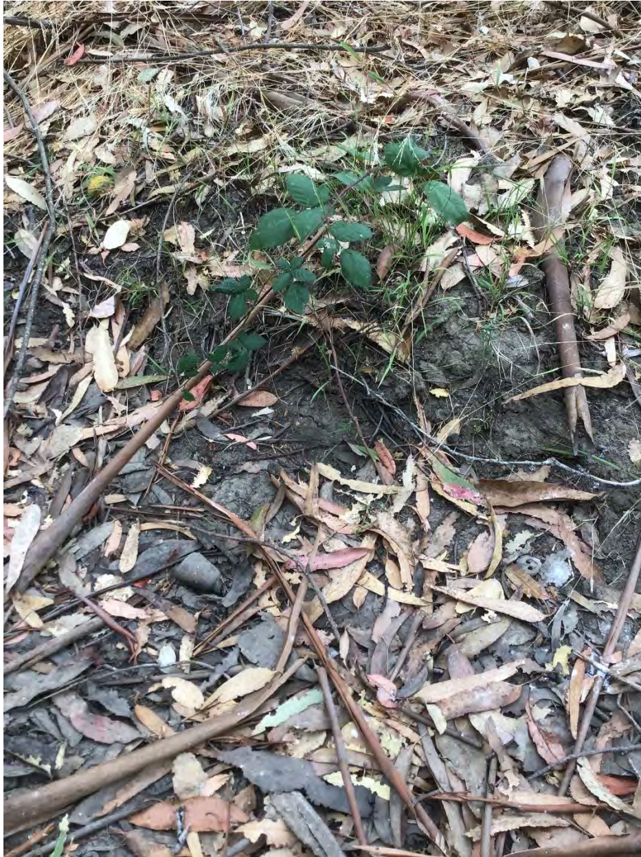
Photo 4. OHWM4 sampling point in ephemeral drainage ES2. OHWM indicators observed included exposed root hairs and roots below an intact soil layer and break in bank.
